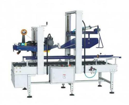
Carton sealers are case equipment that seals the top or bottom of a case with tape or glue. Typically, the minor corrugated flaps are kicked and plowed closed as the cases are transferred. As the cases enter the compression section, the major flaps of the carton are closed and a hotmelt adhesive is applied.
