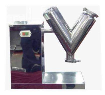
This machine is suitable for pharmacy and other industries, used for mixing the dry granule materials.
