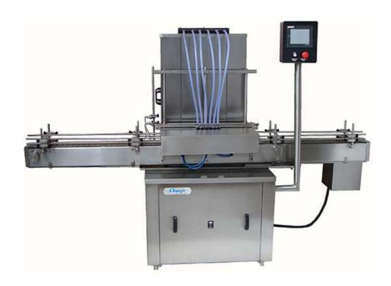
Automatic Accufill Liquid Vial Filling Machine is precision built on sturdy welded steel frame completely enclose in stainless steel sheet and doors are provided to facilitate the servicing of machine. Machine works on VOLUME=TIME TECHNOLOGY AND SPEED=FLOW RATE. The unit is made compact, versatile and S.S. body. No container No filling system arrangement is standard features of the machine. The unit is made compact, versatile and enclosed in stainless steel elegantly matt finish body.
