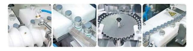
A104 is specially designed for high speed and precision labeling on vials and other small pharmaceutical bottles. Straight line layout and spacing worm are used for easy inline connection. Rotary indexing table aligns vials at three points enabling extra stability and high precision labeling at all speeds. Optional label and code inspection. Patented positive drive rejection wheel mechanism ensures accurate rejection of defective products orderly during high speed operation.
