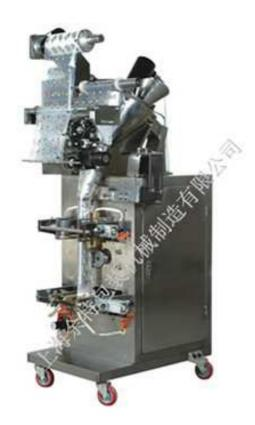
This machine can be to used package non-free-flow products such as powdered coffee, fertilizer, and seasoning, milk powder, medicine powder, and a variety of powders.
