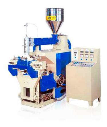
This series machine with special features which is designed especially for producing the drug bottle, toy, Popsicle and etc. This type of machine can produce various material such as PP, PE, PVC. This is the most economical and high performance machinery nowadays.
