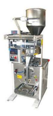
Able to manually complete discontinuous running of forming, filling, counting, printing (it is necessary to separately configure coder), merging functions of photoelectric trace and stepless speed regulation into a single whole with back seal as its seal mode.
