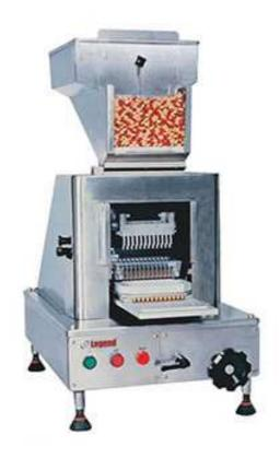
Legend Automatic capsule loader is used in combination with manually operated capsule filling machine where Capsules are loaded in loading tray in cap up-body down position automatically. Our machines ensure higher production at lower cost with better standard of accuracy.
