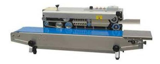
The machine adopts electronic constant temperature mechanism and stepless speed adjusting transmission mechanism. It can seal plastic films with various of materials. such as PP, PE, AlumInum foil, laminated material. And can fixed date embossing system, If necessary, counting device can be fixed to the machine.
