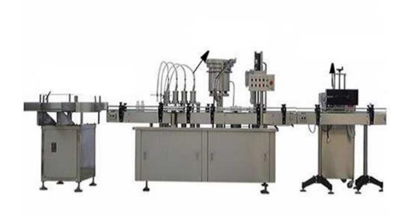
This production line consist of bottle feeding machine, filling machine, screwing machine, aluminum foil sealing machine and labeling machine.
