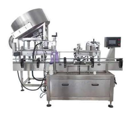
Put all caps into the cap vibrating plate, the cap along the loading cap tunnel placed in the bottle mouth ordered.
