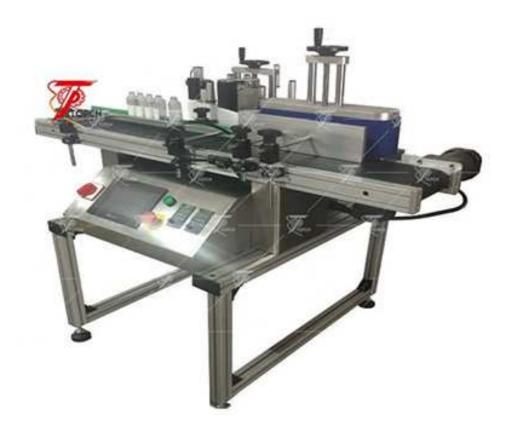
Desktop sticker drink bottle labeling machine has a small footprint, lightweight design, perfectly suitable to use in a small space. Full automatic processing provided by PLC and fast labeling speed to save your precious time, it's the best choice for automatic labeling in a such small factory
