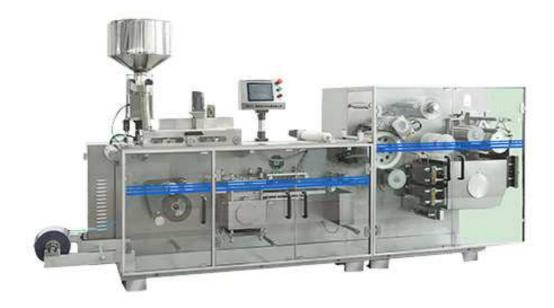
DPH-260 Roller-plate high speed bubble cap packaging machine collected plate type forming and roller sealing as incorporator. It applies to medicine packaging, such as variety specification of sugar coated or uncoated tablet, capsule, soft gel, injection and so on. It's also suitable for packing small hardware, electronical element, medical devices and foods which shapes are similar with above pharmaceuticals.
