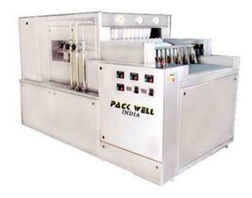
The Pack Well High Speed Linear Bottle Washing Machine is most ideal for Round Bottles and finds wide application in PHARMA, FOOD & BEVERAGES INDUSTRIES. The automatic loading arrangement facilities loading of bottles on to SS wire mesh conveyor through feed conveyor or bottles are pushed manually from feed table. This saves manpower as bottles are feed into pockets automatically. The automatic unloading mechanism consists of unloading bottle continues on to Turn Table.
