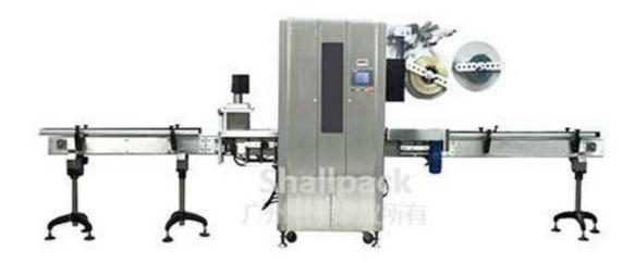
The SL300 Shrink Sleeve Label Applicator can be configured as a full body or mid body shrink sleeve label applicator by simply changing the mandrel and selecting the proper mode in the touch pad control.
