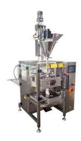
This machine It is suitable for automatic packaging of loose, non-sticky and granular materials such as medicine powder, feed, charcoal, tea, activated charcoal, laundry powder and desiccant, etc. in pharmaceutical, food, daily chemical, pesticide, plastic products and special industries.
