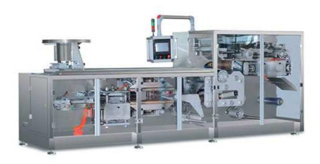
DPH330E Blister packing machine is our company new develop high speed machine which combines the advantage of plate-type and rotary-type machine. With the international high level technology concept, full servo motor, bus control system, modular design, high feeding capacity, intelligent and low noise. Easy operation and mold exchange. Meet GMP quality standard. It is widely used in medicine, health care products, medical devices and electronic components blister packing.
