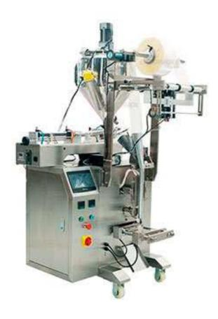
Suitable for packing the fine powder material. Such as coffee powder, spice powder, milk powder, flour, fruits powder, seasoning, chemical medical powder, etc. It integrates metering, bagging, packing, sealing, date printing.
