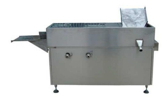
This linear bottle cleaner is the washing equipment of oral liquid production line, and it is mainly used to clean 5-20ml vertical bottles with easy open lids or anti-theft caps.
