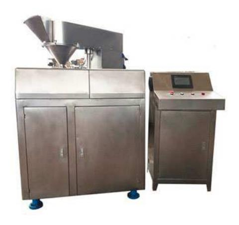
Dryer granulator suitable for laboratory, middle labortary tester and small batch manufacture, it just need 100grams powder into making forming, get request granule, you can adjust granule size and compactness, by PLC control auto control, it will suitable difference requirements, it will improve finish rate, high efficiency, high automatic, easy to use and maintenance, lower noise. Suitable pharmaceutical and food and use daily goods
