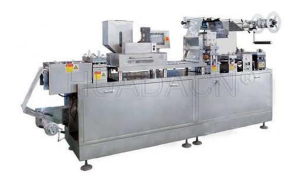
Blister Packing Machine DPP-250 is specially designed for hospital dosage room, laboratory institute, health care product, middle-small pharmacy factory. Featured by compact machine body, easy operation, multi-function, stroke adjustable, long durability etc, it is suitable for the Alu-PVC package of medicine, food, electric parts etc. It has aided forming Pre-cutting Inspection and rejecting control systems, with print mark registration Automatic feeder.
