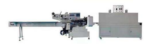
It works from feeding, bag forming to sealing and shrink wrapping, widely used in food, medical, cosmetic and stationery industry.
