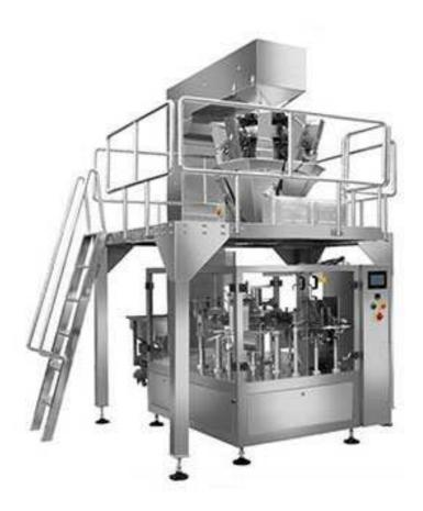
This packaging machine adopts a multihead weigher for weighing and measurement, and various numbers of electronic scales are available for selection according to the packaging materials and speed requirements. The loading mechanism adopts a bucket loading machine, which has the functions of automatic filling of material shortage and automatic stop when the material is full.
