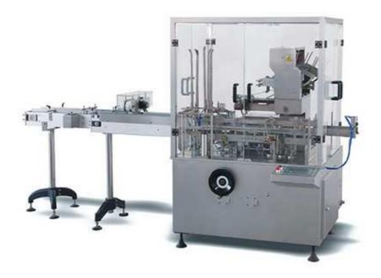
The equipment is mainly used for automatic packaging of injection drugs in trays or injection in bubble cap board trays and similar specifications' items, and if it can connect the front printing equipment or equipment of making trays connecting printers, this will improve productivity.
