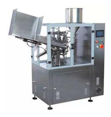
Automatic plastic tube filling and sealing machine is suitable for filling material into the plastic tubes, then seal the tube.
