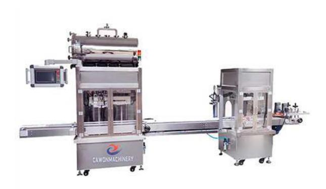
This automatic filling machine is with larger air cylinder which can help to fill liquid faster. This machine is easy to operate and each nozzle can be controlled separately, it can work with the capping machine, labeling machine to achieve to automatic production.
