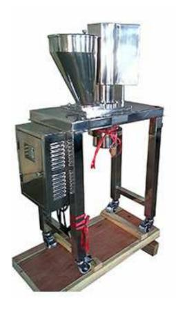
FZ series grinding and granulating machine is used in pharmaceutical, food, fine chemical processing industries. This machine reaches the world advanced level and conforms to the GMP specification. It is completely made of stainless steel material.
