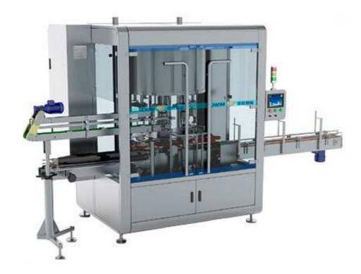
The machine integrates bottle inlet, cap feeding, screwing and bottle outlet. It uses the cap grab and positioning capping. The whole machine is rotary structure, suitable for the capping of pump cap and sprayer cap. In the process of capping, there is no bottle damage, cap damage phenomenon, high efficiency of capping, high qualified rate, stable operation and wide range of use.
