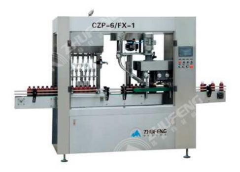
The machine is a two-in-one full-automatic filler integrating in filling and lid-revolving, usingastospheric timing filling and single-head intermission positioning lid-revolving, it suits for the dividing filling and sealing of all kinds of bottle shape for the daily chemicals, foodstuff, pharmacy, chemical industry and pesticide. It has PLC program control, filling speed fast, operation simple and convenient, measurement accurate, and high acceptance rate of lid-revolving, long use lifespan.
