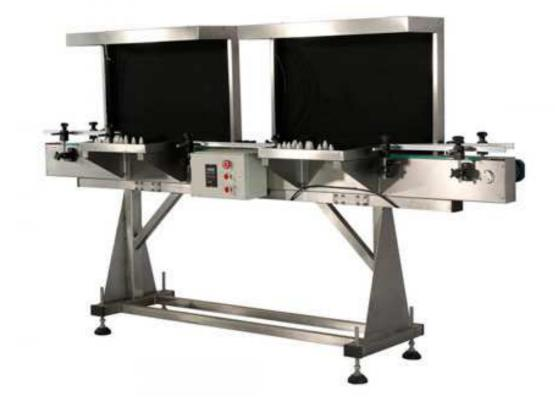
The light inspection machine is specially designed and manufactured according to whether there are defects in the appearance of the bottle after filling. By using LED irradiation on the bottle body, black and white background comparison, operators can clearly see whether there are defects on the outside of the bottle after filling, so as to carry out screening and removal.
