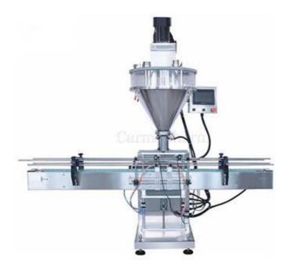
This Auger Powder Filling Machine is mainly used for weighting powder materials. It adopts screw quantitative and manual feeding. The machine structure is simple, it is very convenient for operation and cleaning. The dust is small in the production process, high in efficiency, very timesaving and labor-saving. It is the most commonly used in powder packing industry. The packaging method with the screw feeding are more precise and convenient.
