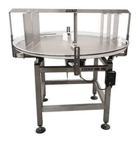
Constructed from high quality stainless steel materials with variable speed drives, reversible rotation and height-adjustable features, SureKap Unscrambling Tables are designed to help your system operate at its maximum efficiency. These turntables allow for the loading of bottles to conveyors with ease.
