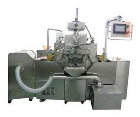
This machine is the absorption of advanced technologies at home and abroad, based on a combination of soft capsule production process and the characteristics of the use advanced technology and high quality materials. Meet the GMP requirements of well-designed. This machine consist of soft capsule machine, sol pot, mould (die roller), capsule conveyor, tumbler dryer, cooling air machine, vacuum pump, drying tray, vacuum mixing barrel and electrical control system and other ancillary equipment.
