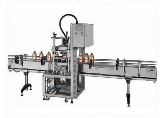
Zhonghuan Company offers a variety of screw capping machines (rotary capping machines) for a number of different industries and products. The high speed bottle capping heads provide for repeatable and reliable cap application of the screw caps. The rotary cappers use presorted caps that are picked up and secured and then placed on the containers.
