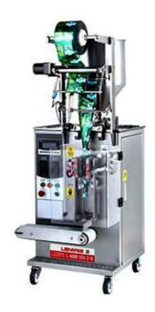
Automatically making bags, weighing, counting, filling, sealing, cutting
