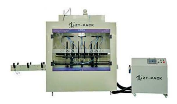
This volumetric piston filler is a type of corrosive filling machines specially designed for automatic filling of caustic liquids such as toilet cleaner into bottles. This piston filling machine is suited to fill low viscosity liquid into bottle with capacity of 500ml-5l, bottle diameter of 40-150mm and bottle height of 80-370mm. It can be changed to different bottle sizes without any tool, and can be easily cleaned by using water.
