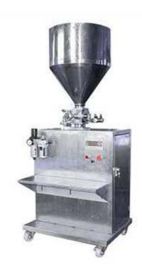
Be suited for various fluid and semi-fluid in food, medicine and chemical engineering Filling of 100 ~1000ml/cycle measured by cock pump volume method as fitting various container to filling head manually. Stepless setting of cycle number and no limit filling amount. According with the heath standard. Stirring unit for the users' order.
