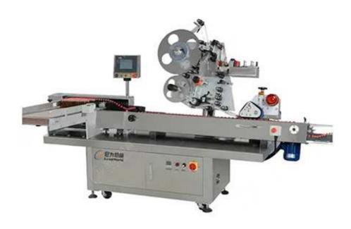
KL-800 main parts would be labeling head, stainless steel 304 frame, conveyor system, sponge pressing while and Siemens PLC touch screen and servo motor for fast speed labeling.
