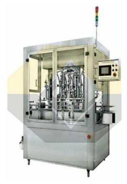
VFO-6M Automatic 6 Heads (Piston) Oil Filling Machine (Motor Control) aim to oil realm such as lubrication, edible oil etc, and other realm like agrochemical. It is suited various figure containers. The filling volumes range is 1L-5L, the max filling speed can reach 3000 containers/hour for 1L.
