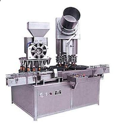
SBPF-MR100 Automatic Monoblock Dry Syrup Powder Filling with Eight Head ROPP Cap Sealing Machine is a Compact machine used for filling and sealing of Dry Syrup in bottles.
