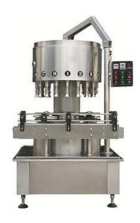
Filling of liquor, wine, fruit juice drink not containing gas, such as can also with vinegar, milk, liquid filling in such as pesticide, has not broken bottle, no drip, operation and maintenance is convenient wait for a characteristic, and is equipped with overload protection and liquid crystal display device. Because of the filling in the closed area, the pollution and the spread of harmful substances can be eliminated, which meets the requirements of the food hygiene law.
