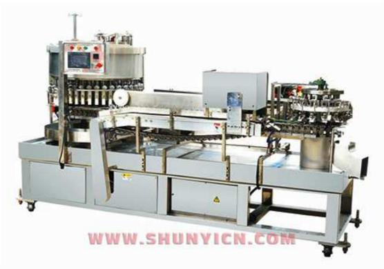
The machine is suitable for filling and sealing for the products made of LDPE, such as ice loll, (grenade, corn, banana, rabbit etc) toys jelly.
