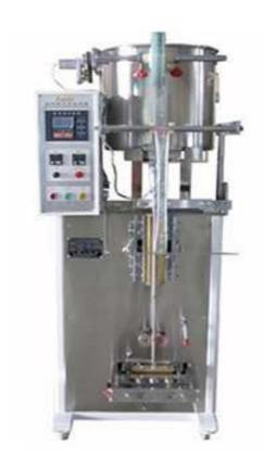
It is specially for packaging fruit jelly, ice, drinking, oil, and yogurt bar or stick. Automatically packaging, measuring, stuffing and cutting.
