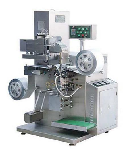
This machine adopts variable frequency speed regulating, vibration blanking mechanism, material quantity photoelectric monitoring device and automatic filling. Such production processes and assemblies as heat-sealing, line cutting, batch No. printing, cutting and automatic counting, etc. have been automatically finished.
