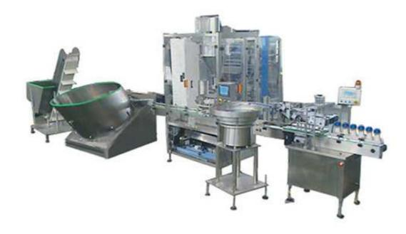
This filling line is a highly automatic and intelligent bottle/can filling equipment developed by our company, which consists of four parts: bottle loading machine, bottle sorting machine, filling machine and capping machine.
