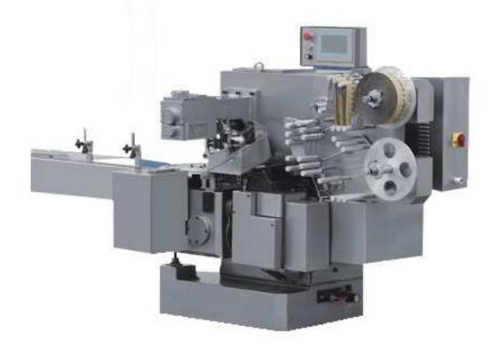
DWC300 Double Twist Chocolate Packaging Machine is designed for high speed packing chocolate & candy into double twist style. Chocolate or candy which are unfit for automating arrangement were feed by conveyor belt, then to be auto pushed into feeding plate by mechanical. Film length change by PLC. Machine of modern design, easy to clean and easy for maintenance. The customized machine also be connected to bowl feeder or aligner feeder according to different products.
