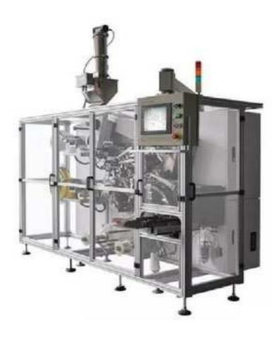
The machine SP-100SN is a kind of automatic tea bag machine for the packing of tea and similar Chinese herbs / Flower tea. It makes double chamber tea bags which are cold-sealed. The machine links up hard label and thread with staple, and the tea bags are pushed out and packed into box manually after counting. The packing materials are non-heat-sealed filter paper, label, thread and staple.
