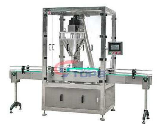
Automatic auger filling weighing machine is an updated rotary type fill-by-weight automatic auger filler. It is a Filling-by-Weighing auger filler developed by Vtops Machinery for high-end customers with High-Precision needs. The filled error of the auger filling weighing machine is less than 1 gram.
