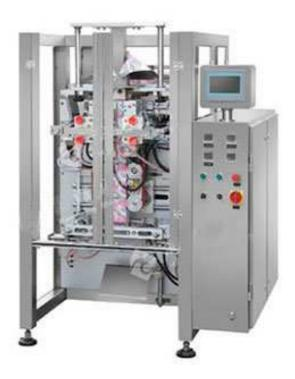
The machine is suitable for measuring packing irregular solid and granular and powder materials, such as candy, biscuit, dry fruit, coffee beans, sugar and milk powder, protein powder, rice flour, starch seasoning powder and so on.
