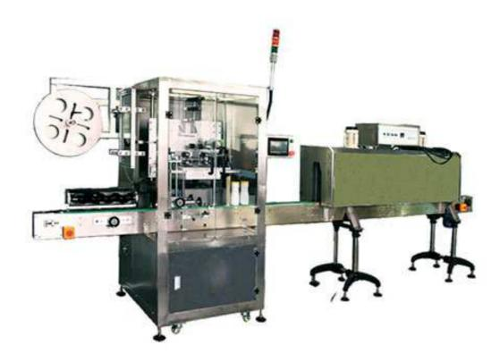
The round bottle, the square bottle, the oval bottle and the pillow type bottle sleeve are contracted, and the bottle mouth, the bottle body and the surrounding product sleeve can be set. It can be used stand-alone or connected to the production line.
